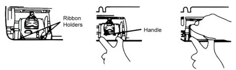
3. Correctly insert a new cartridge between the ribbon guide and the printer head.
